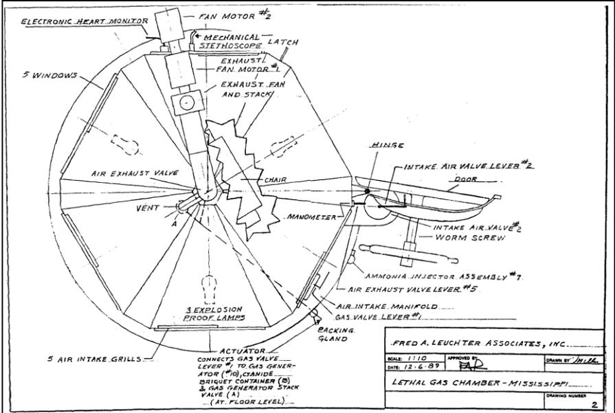
Fig 83 & 84: Technical drawings of the Parchman (Miss.) execution gas chamber.
